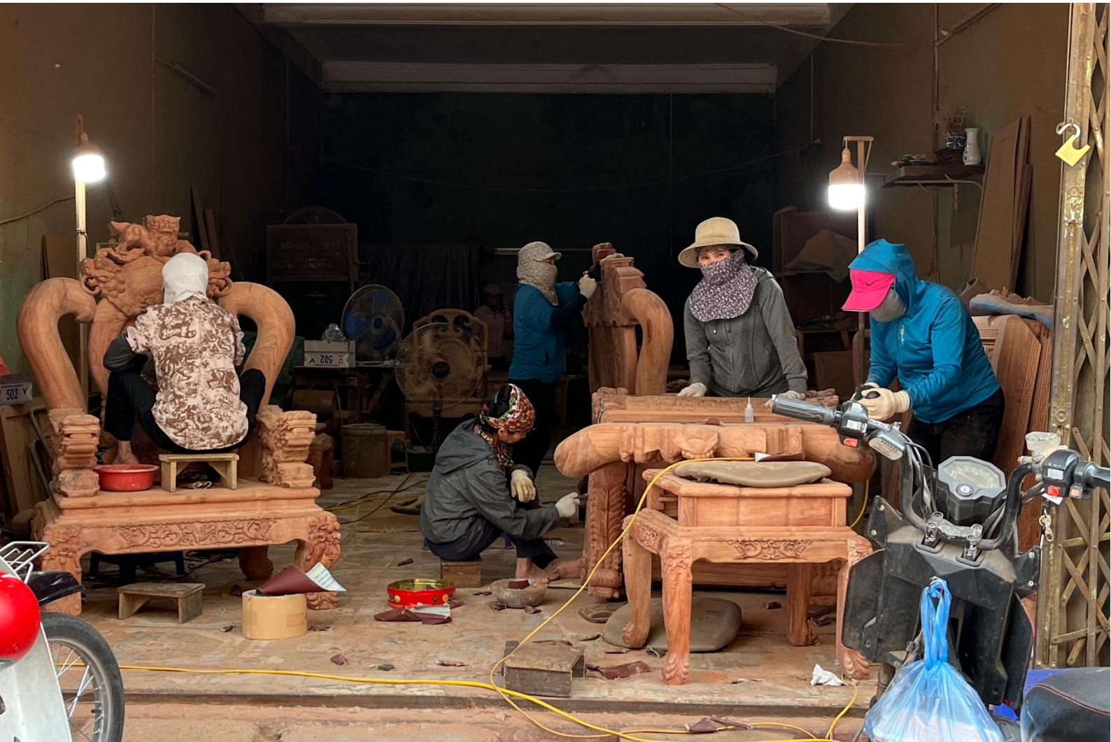
Photo 3: Female workers sanding wooden furniture in Dong Ky craft village. Source: Forest Trends
