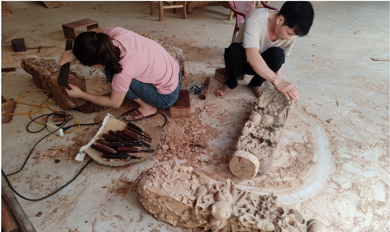
Photo 4: A household is carving and finishing an altar table leg in La Xuyên craft village
